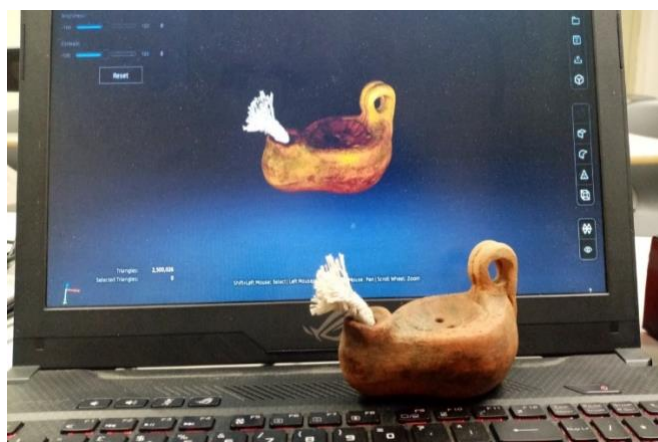
Figure 1. Replica of a Roman oil lamp, 3D scan made at Lab-H of the University of Salerno using EinScan-SP by Shining 3D .
